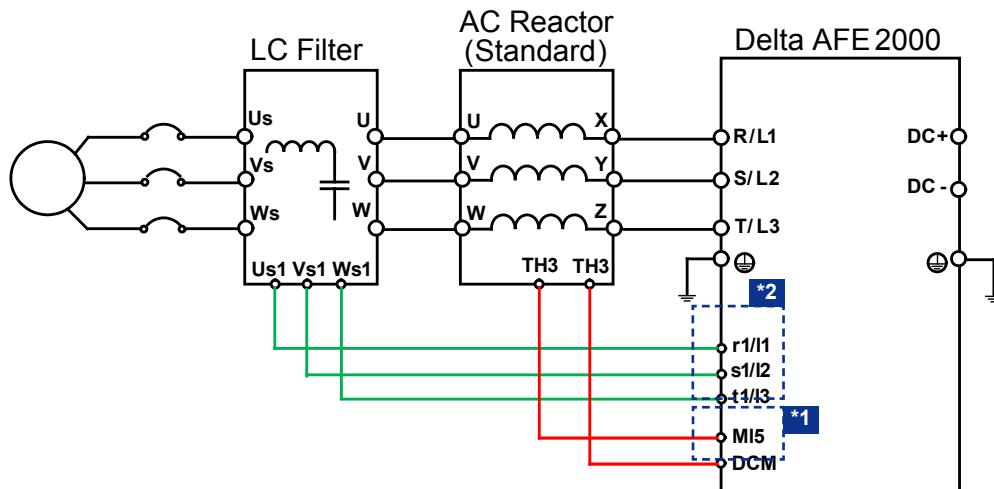
\*1 Delta's AC reactor (standard installation accessory) is equipped with a thermal protection function. The TH3 terminal will have the AFE2000 send out a warning message when the reactor temperature exceeds 120°C .
