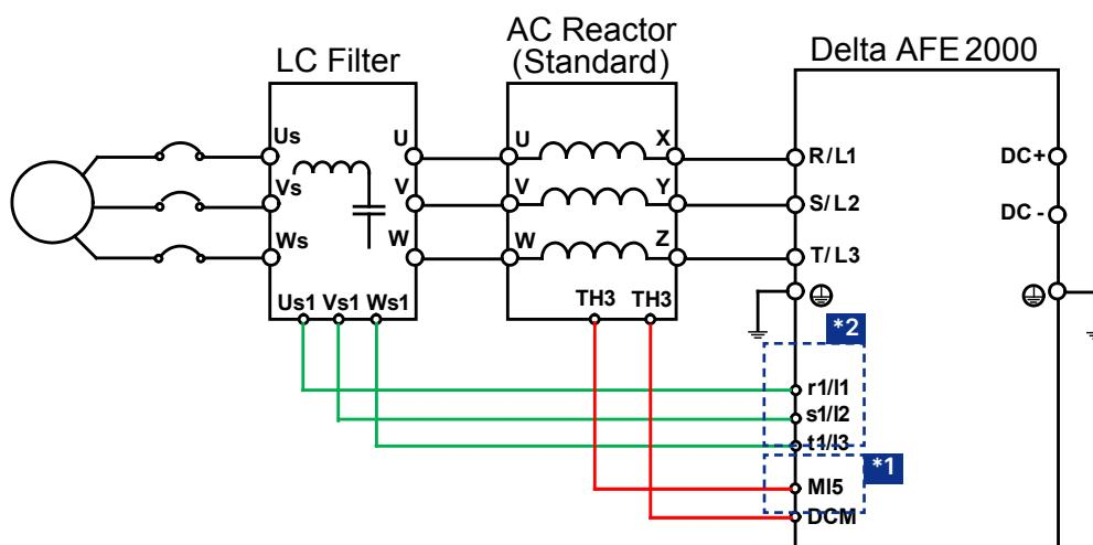
\*1 Delta's AC reactor (standard installation accessory) is equipped with a thermal protection function. The TH3 terminal will have the AFE2000 send out warning message when the reactor temperature exceeds 120°C .
