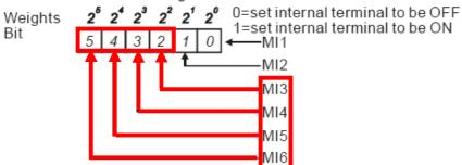
Change the status of bit2 - bit5 to set the multi-step speed command, and trigger the different bit status which wrote in the macro of button.
