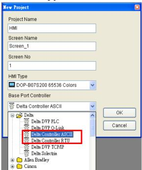
Use one of DOP-B type, the base port controller can be selected as Delta Controller ASCII or Delta Controller RTU.
