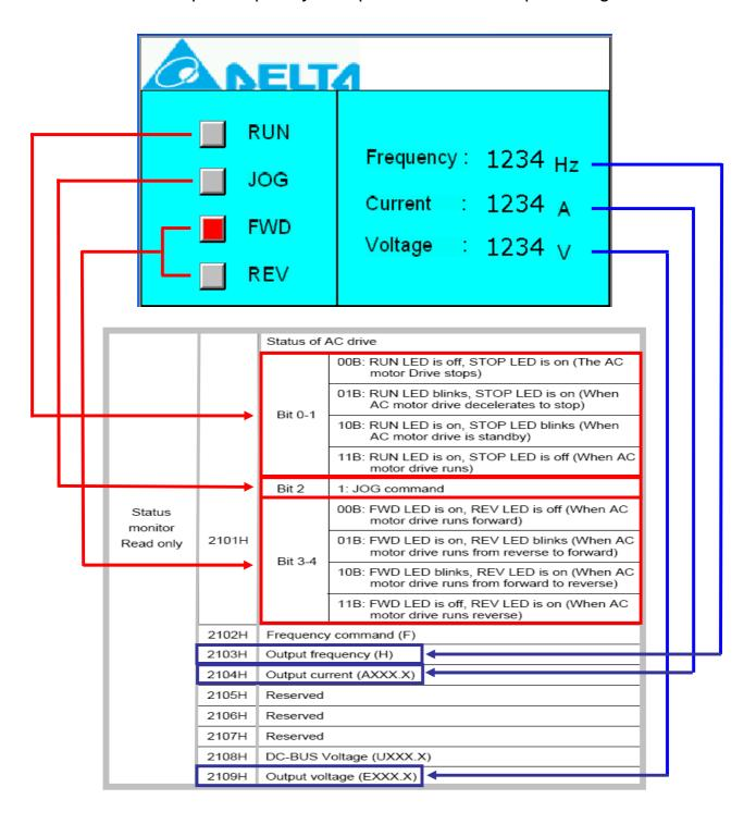
Edit the macro in Screen Cycle Macro  $\,^{,}$  and use the bit of 2101H to monitor the status of AC drive  $\,^{,}$
