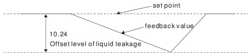
When the rate of change of feedback value is higher than [Pr10.25/Pr10.26], it is assumed the leakage is too fast or there's more than just liquid leakage. When the system is in constant pressure status, the VFD-EL will start to run if this is the case.
