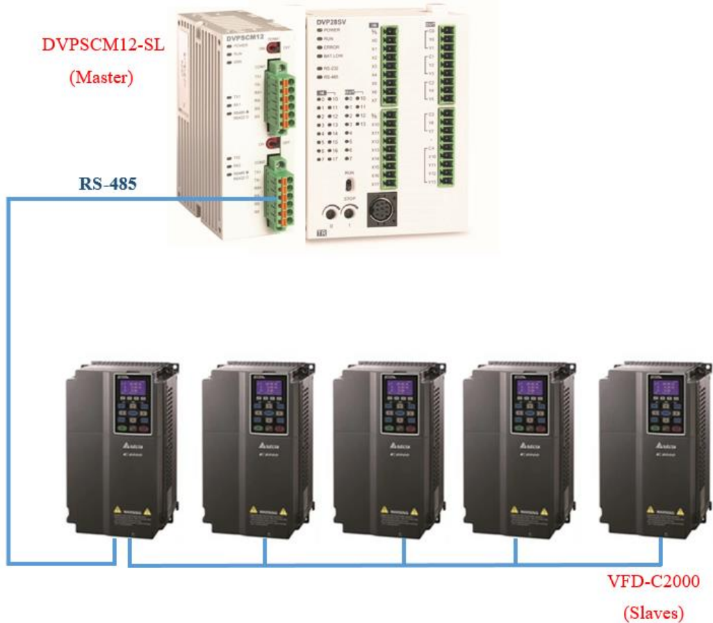
Figure 3: DVPSCM12-SL as Modbus Master and VFD-C2000 as slaves
