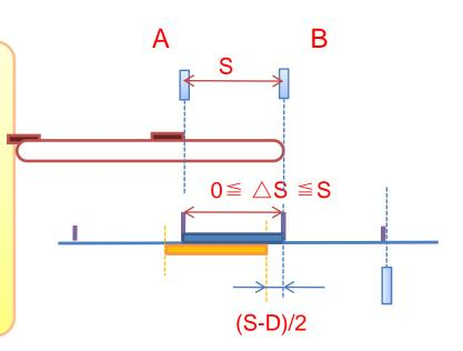
ightharpoonup The blue section is the area of chain hook ,and the orange is the area of target line which always fall behind the chain hook (S-D)/2 .
