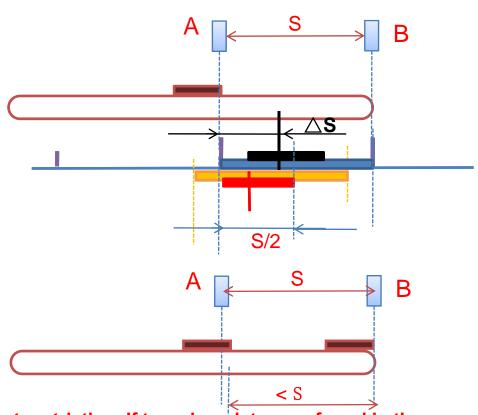
Without restriction, If two chocolates are found in the same time of "T", the next one is likely to cause that the servo drive may accelerate too fast, and the first one may have large position deviation. On the individual adjustment belt, there may be the appearance that two chocolates are catching up the same target line, and it easily cause both of the two chocolates being sent into the same chain hook. Therefore, the chocolate should decelerate to wait for the next target line.
