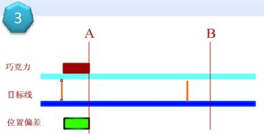
If chocolate is not much behind the target line, it should accelerate and catch up the line.
