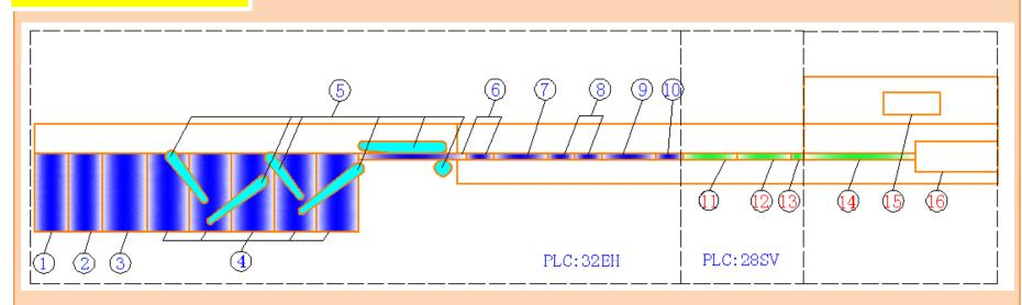
$1\sim10$ : ten VFD-M AC motor drives
